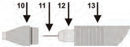
Lightly rotate the nozzle (10) back and forth and in doing so, pull it off of the handpiece (13). It is only pushed-on, not screwed in place.
