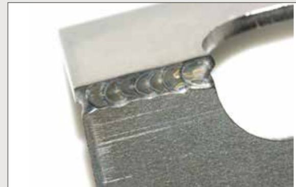
Weld seam on a workpiece made of Hastelloy
