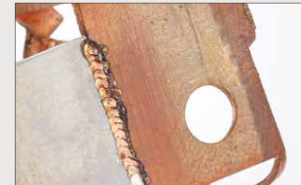
Material mixes of different alloys are possible. (Photo showing stainless steel and copper)
